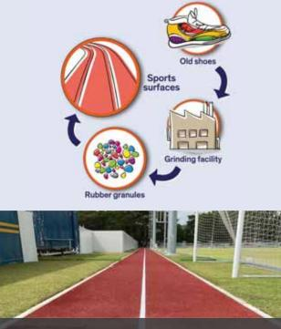
(Top) Process behind repurposing the old shoes and (Bottom) 108m running track built using recycled rubbers granules
